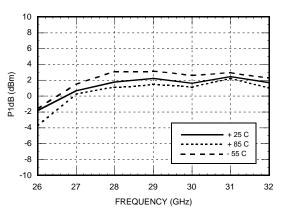
Input P1dB vs. Temperature @LO = -5 dBm, Vdd = +3V
